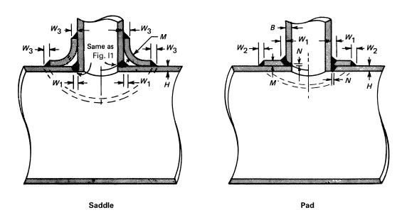
$W_1$  min. =  ${}^{3B}\!/_{8}$ , but not less than  ${}^{1}\!/_{4}$  in.  $W_2$  min. =  ${}^{M}\!/_{2}$ , but not less than  ${}^{1}\!/_{4}$  in.
